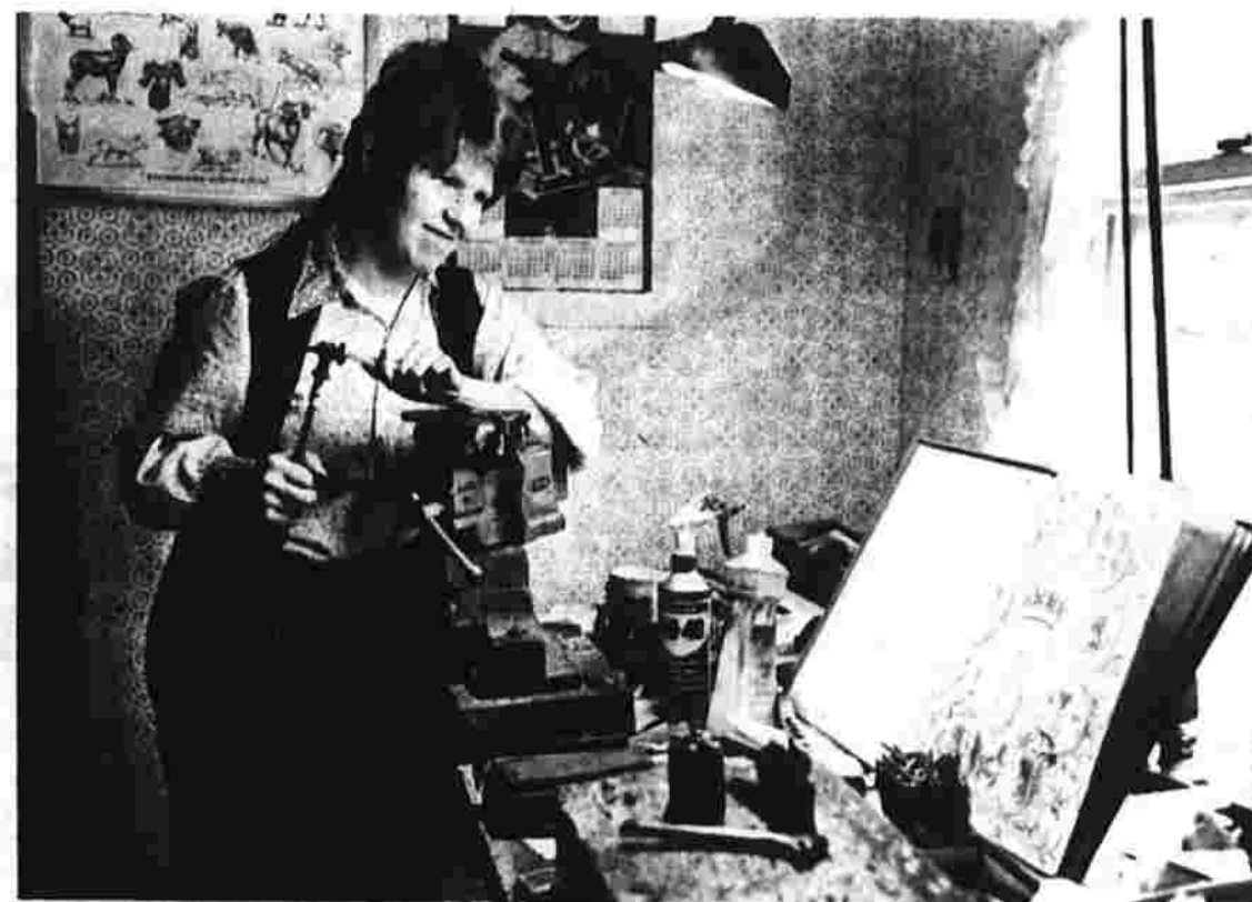
Denise Thirion studies a design which she is reproducing by engraving on the stock of a hand gun. With quick raps of the hammer on a delicate chisel held in her left hand, the design takes shape.
